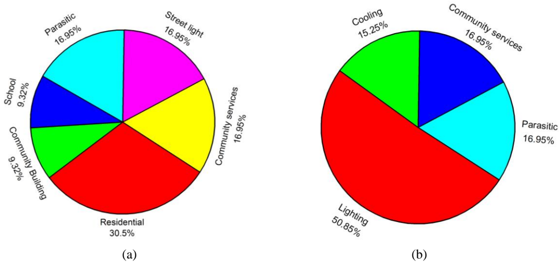
Figure.1 Relative load distribution with respect to the (a) utility sector (b) application
