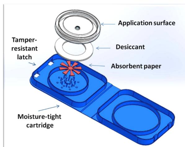
**FIGURE 1** The HemaSpot blood collection device showing the blades of the fan-shaped filter paper (in red). Once blood has been applied through the hole in the application surface the device is folded over and snapped shut. Image courtesy of Spot on Sciences.
