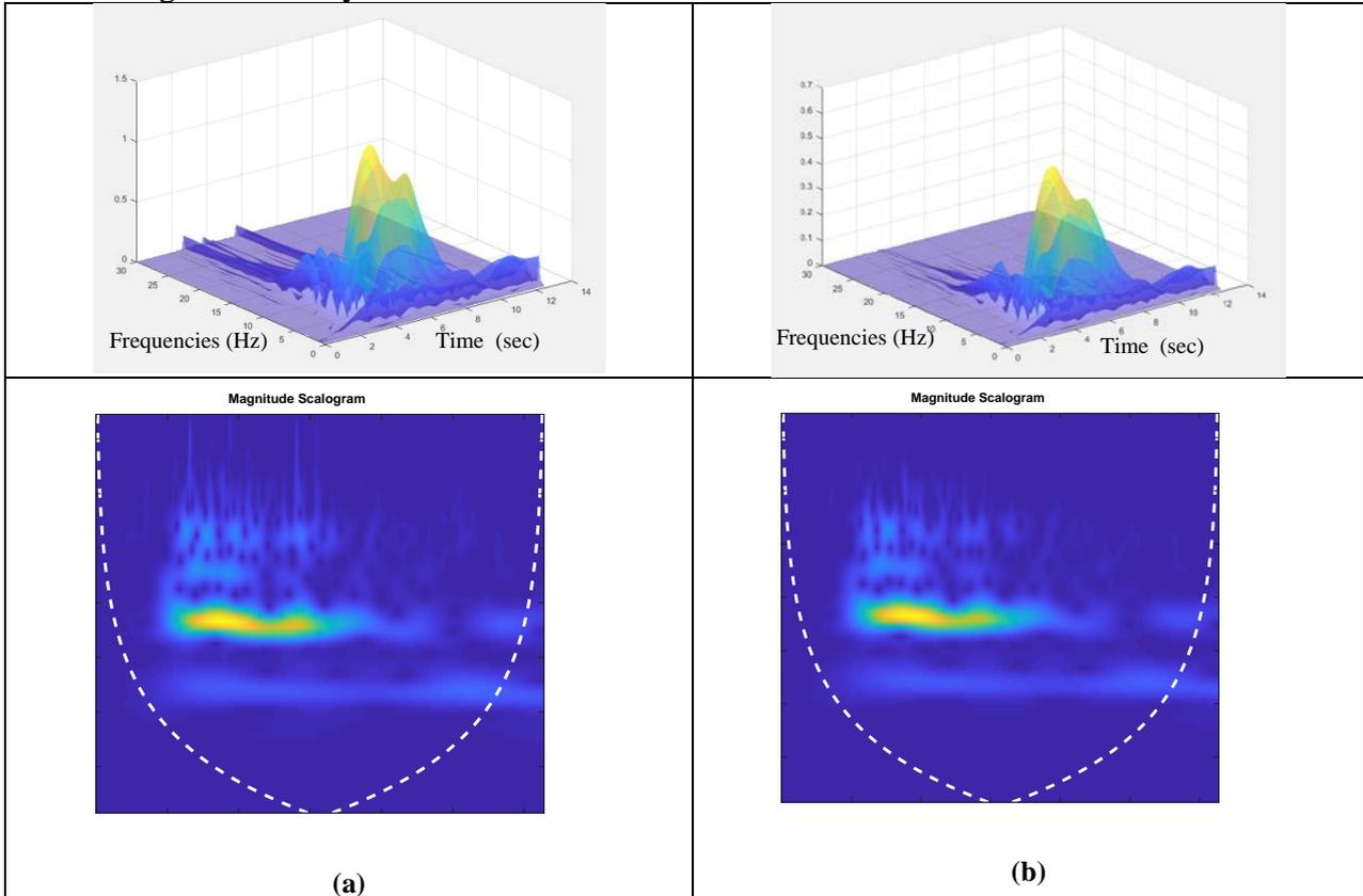
Figure 4: Continues wavelet transform from response measured at 1st floor for healthy (b) and damaged (a) frame.
