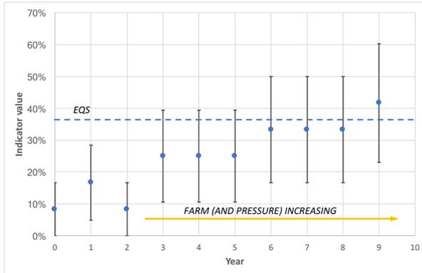
Figure 6: Uncertainty in measurement. (Figure 1 revisited.) Each estimate of an annual value of  $S$  includes a confidence interval: according to normal statistical practice, 19 out of 20 resamplings of each  $S$  would be expected to fall within the corresponding vertical bar. When does the time-series first transgress the EQS?
