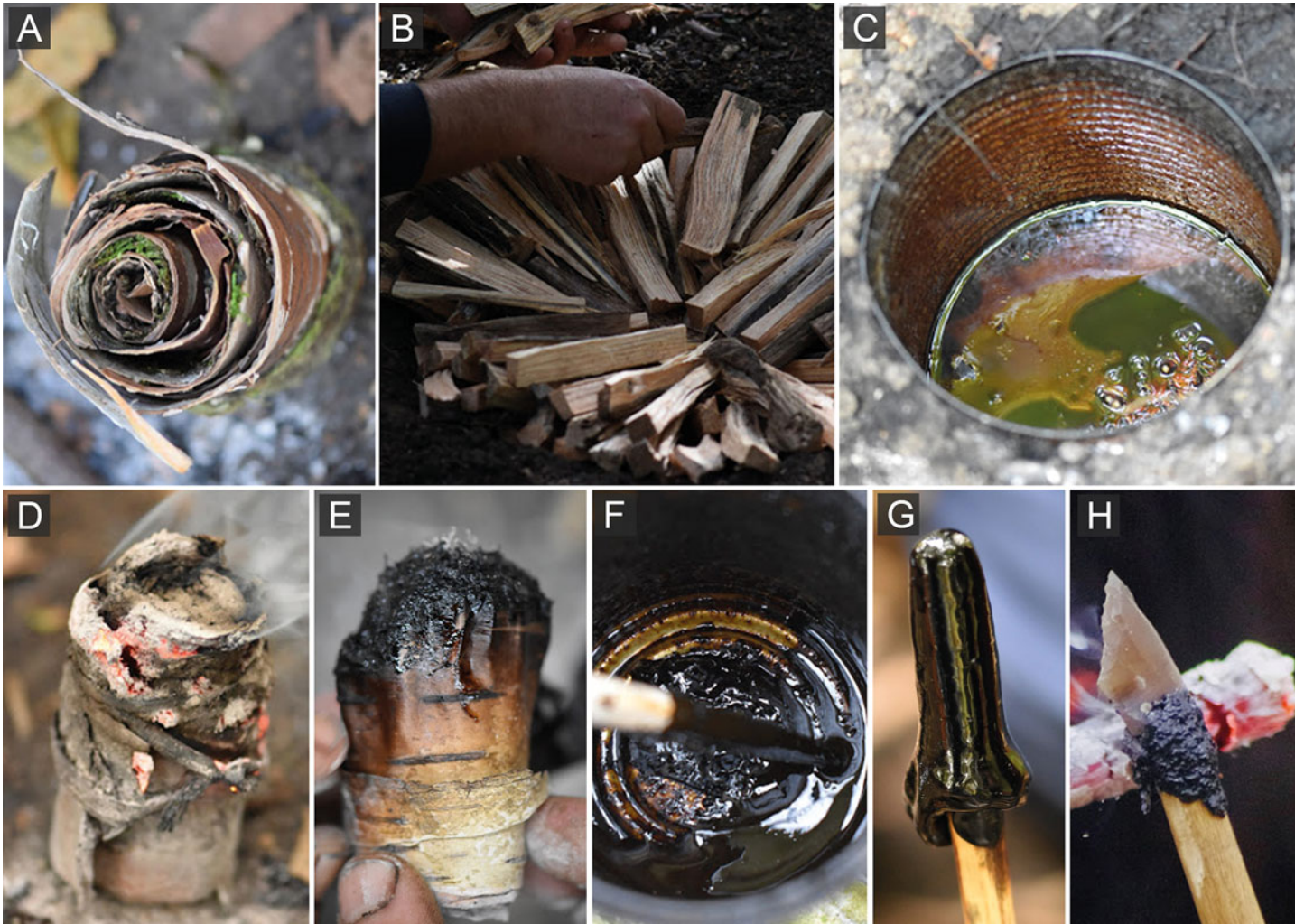
Figure 1. (A) Rolled birch bark; (B) aceramic pine-tar production; (C) aceramic yield of pine tar stored in a metal container post-production—turpentine, one of the pyrolysis fractions of pine wood, displays iridescent ‘rainbow’ effect; (D) roll of birch bark still burning post-use in aceramic production of birch tar; (E) birch bark undergoing phase-change from solid to liquid; (F) reflective and glossy yield of aceramically produced birch-bark tar stored in metal tin; (G) a tar stick—useful for storing, transporting and reheating tar; (H) tar on a projectile is heated to make it malleable for moulding into desired form. (All photos © YEAR Centre.)
