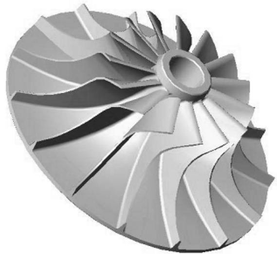
Figure 15. Three dimensional solid model of the designed impeller.
