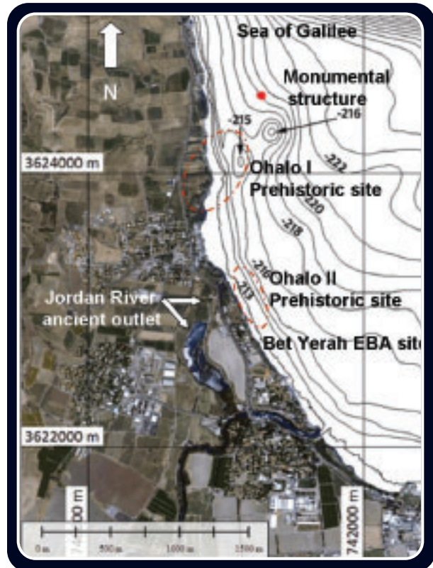
The lake bathymetric map based on a multi-beam survey with the location of the monumental structure (red)
