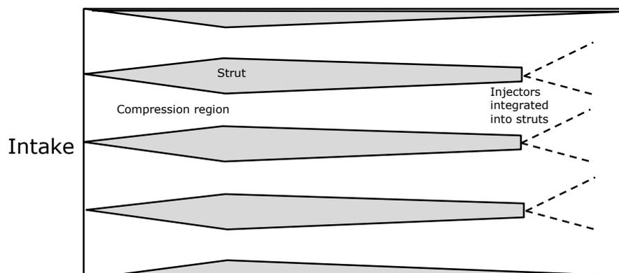
Figure 4, Intake of Strutjet engine, plan view.
