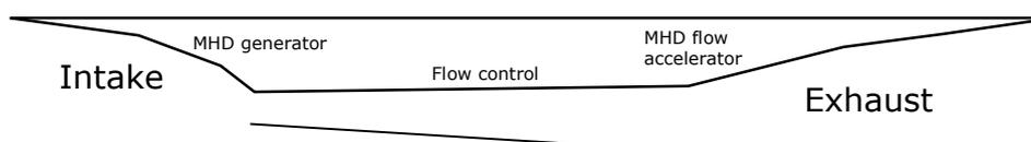
Figure 5, Use of MHD in Scramjet-like systems.
