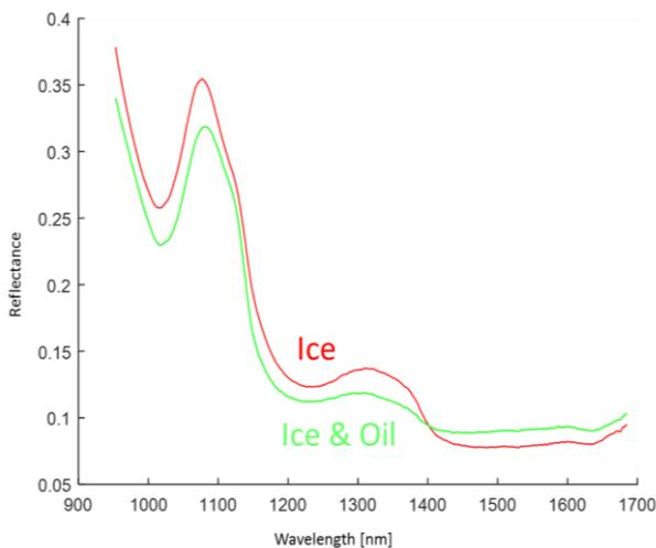
Figure 3. Spectral response of pure ice and ice with oil underneath
