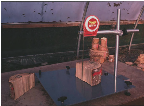
Figure 2 Split disc and the apparatus used for measuring grain angle.
