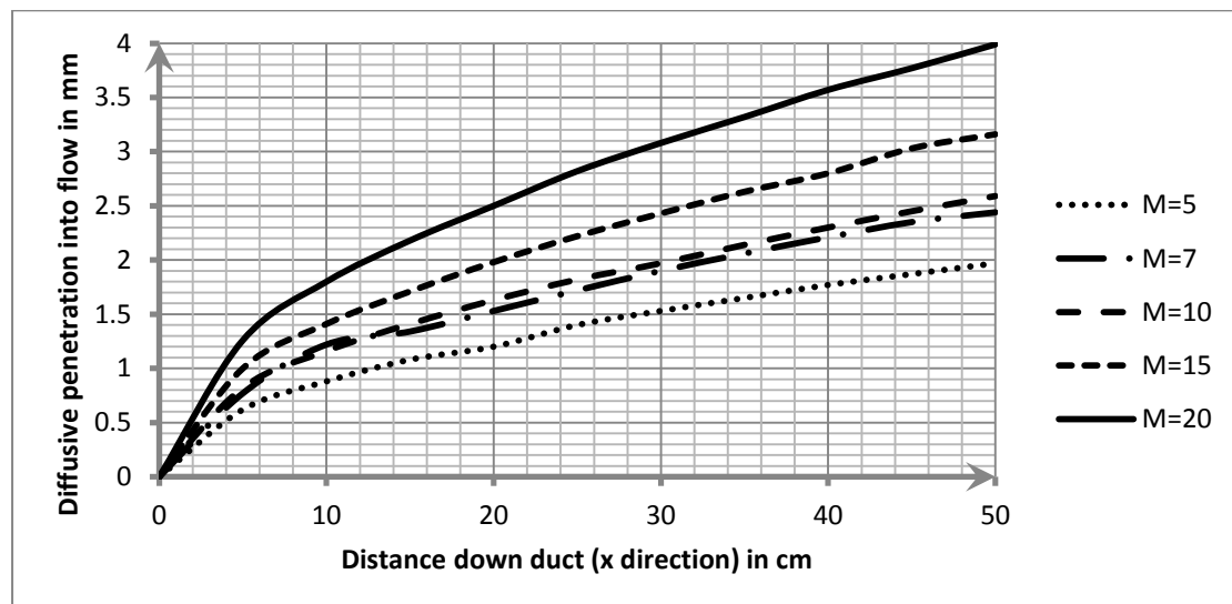
Graph 1, Penetration of fuel into air-flow at various free-stream Mach numbers.
