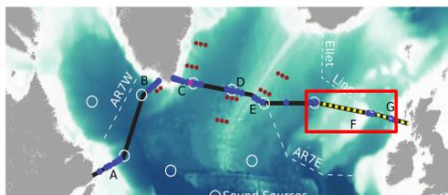
Fig. 1: The OSNAP line, comprising: 1) German (A), US (B,E), US/UK (C), Netherlands (D), UK-SAMS (G) mooring arrays; 2) UK-SAMS glider survey (F); 3) US floats (red dots) and sound sources (white circles)
