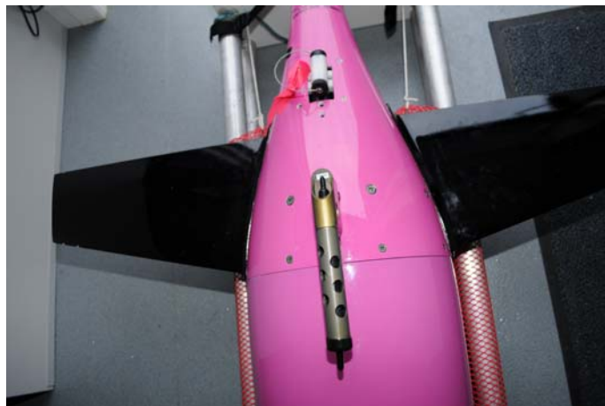
Figure 1. The Sea-Bird sensors. The temperature-conductivity sensor package is directly above the wing. It has protective end caps in place.
