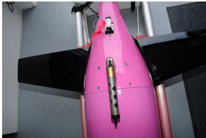
Figure 1. The Sea-Bird sensors. The temperature and salinity sensor package is directly above the wing and the DO sensor is in the short white tube slightly behind the wing. Both sensors packages have protective end caps in place.
