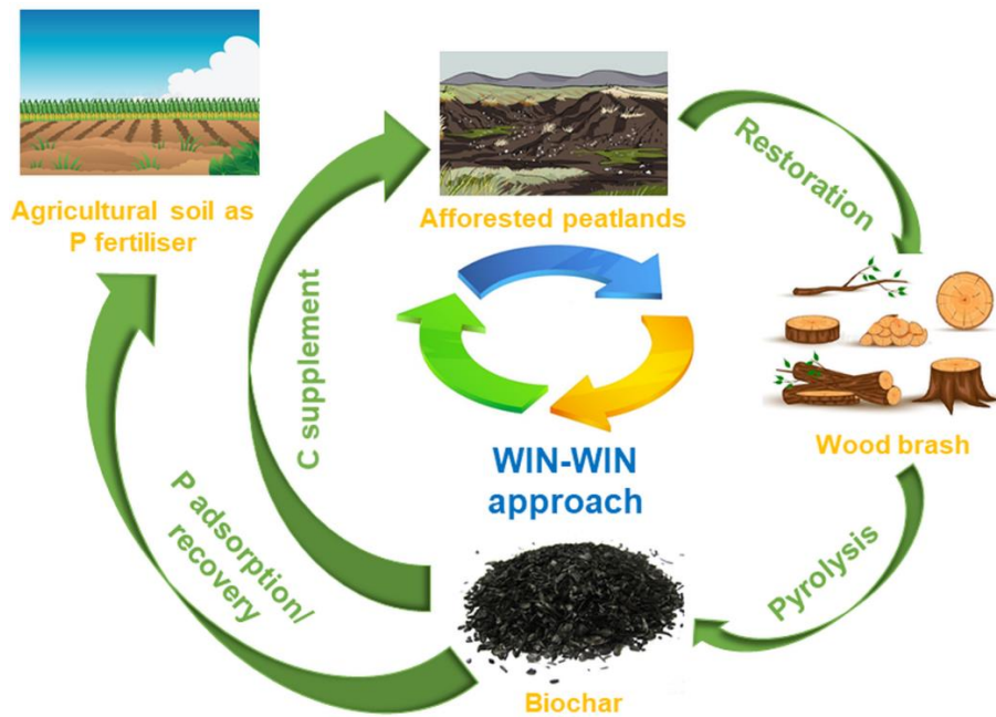
134 Fig. 2. ‘Circular economy’ based approach – involving the utilisation of waste wood 135 brush (created following tree felling during peatland restoration) to create a biochar 136 that could then be P-enriched and used as a fertiliser in new forestry (or remain as a 137 soil C stabiliser)
