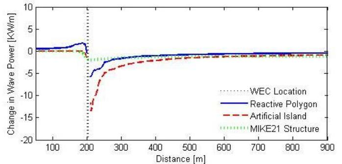
Fig. 6 Change in wave power along the perpendicular transect where  $y = 500$  for each method of modelling a device presented in Fig.5.
