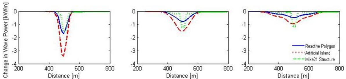
Fig. 7 Change in downstream wave power for device parallel transect downstream of a single device where (left)  $x = 300$ m (middle)  $x = 500$ m and (right)  $x = 700$ m behind the device. Corresponding to 100m, 300m and 500m behind the device.
