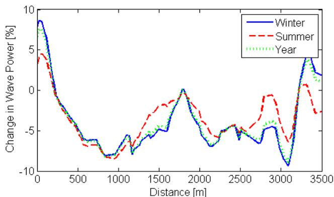
Fig. 15 Change in wave power 300m behind the array for a device parallel transect.
