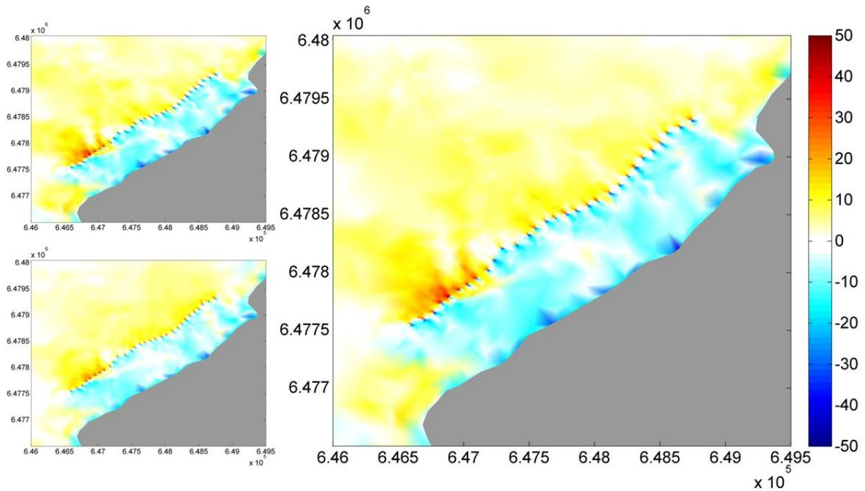
Fig. 13 Percentage change in wave power behind multiple Reactive Polygon structures in UTM-29 coordinates. Top left: winter average, bottom right: summer average and right: yearly average.
